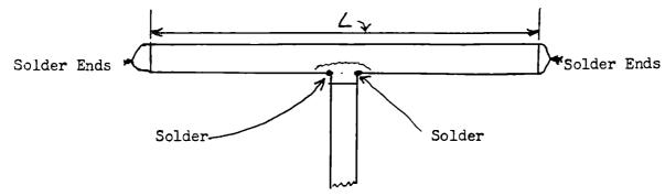
For best results the antenna should be mounted as high as possible and in the clear away from trees, power lines and other surrounding objects. Standard glass or porcelain type insulators can be used on the ends for support and in the center where doublet type antennae are used.
