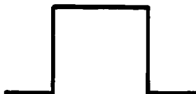
Fig. 11. Illustrating optimum high-frequency response as a result of correct probe adjustment.
